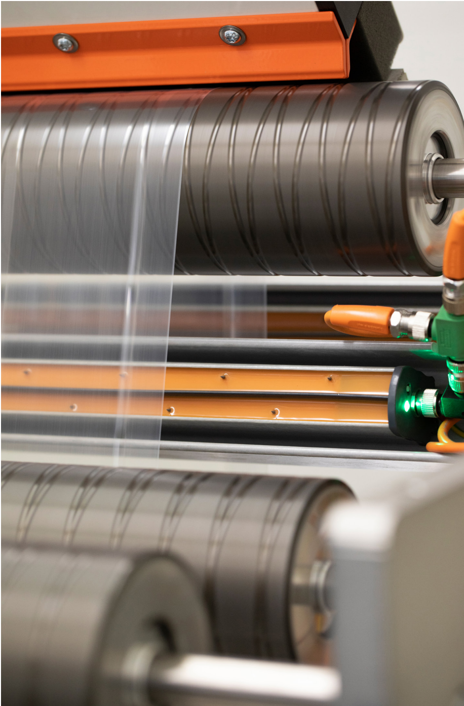
Electrostatic discharge with iONstream 4.0 and AUTO DC technology
