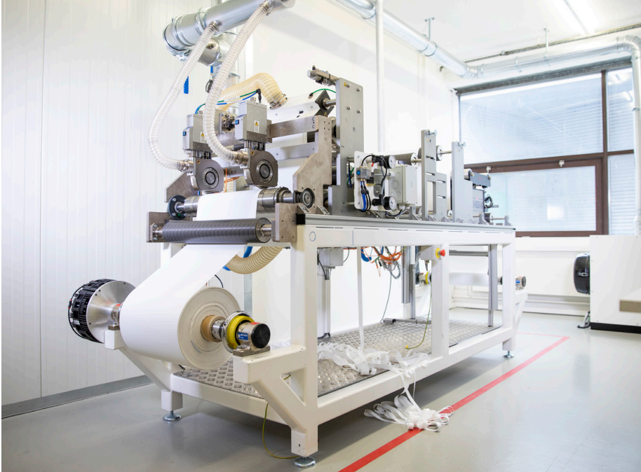
The laboratory facility at Gema with the SLITstream slitting dust extraction system
