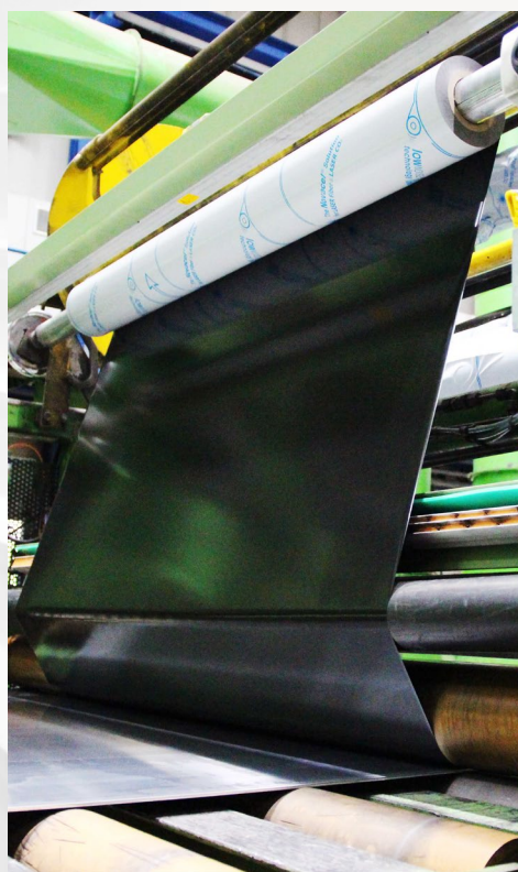
2x iONstream FUSION, 6kV, 2120mm Antistatic bars
