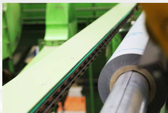
2x iONstream FUSION, 6kV, 2120mm Antistatic bars
